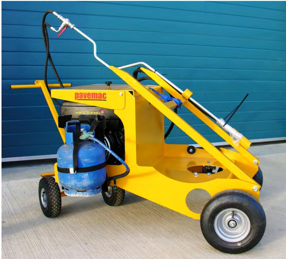
Hatz Diesel Engine 6HP - Mechanical Single Lever Industrial Clutch
