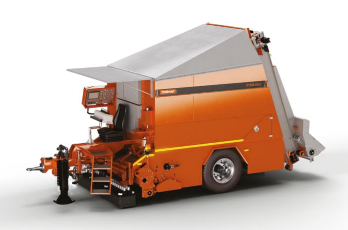
Strassmayr R 7500 Vario is a surface repairing machine assembled on a single-axle trailer. Thanks to its big aggregate hopper and an external emulsion connection, it is able to perform larger jobs on long distances. The whole process of reparation is controlled by a computer, ensuring even distribution of both materials independently of the speed of the carrier truck.
