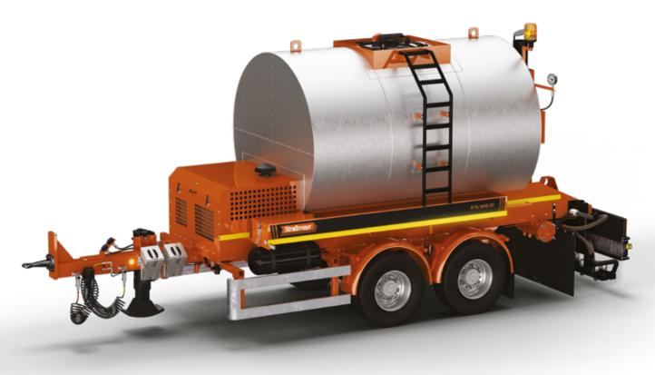
The RTS EF series sprayers are built on one or two-axle chassis and are used to evenly spray the roads with emulsion or serve as a stationary tanks. These machines can work independently of the towing truck, tractor or a tip-car. Emulsion is kept in an isolated tank and automatically heated by a light oil burner controlled by a thermostat.
