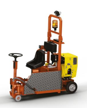
The Strassmayr S FF milling machines are used to prepare expansion joints or clean the cracks before application of special sealing compounds. Hydraulic drive of these compact and robust units allows easy and comfortable work. The steering wheel is directly connected with cutting tool, which allows smooth cutting regardless of the complexity of the course. Foldable protection of the operator and seatbelts secure the safety of the operator.
