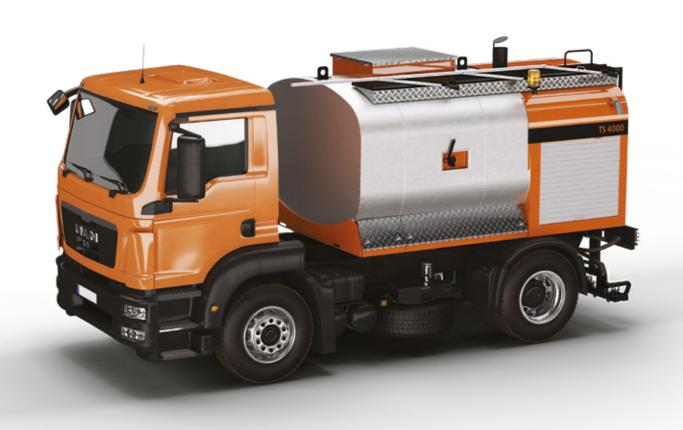
Strassmayr manual sprayers are prepared to be mounted on a truck chassis, with tank sizes from 4 m³ up to 6 m³ and are meant to achieve the same target: even, quick end effective spraying of asphalt emulsion. Automatic temperature control ensures the emulsion is kept always at the desired temperature range.
