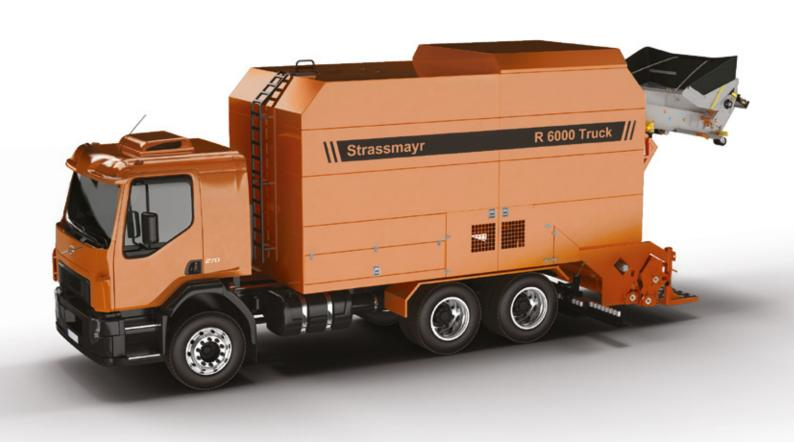
Strassmayr R 6000 Truck is a machine designed to perform large area road surface repairs, using emulsion and grit technology. The unit is built on a truck chassis or in a form of a semi-trailer allowing high manoeuvrability. The process of spraying the surface with emulsion and simultaneous application of aggregate is controlled by a computer, which is responsible for the precise dosage of both materials independently to the speed of the carrier.
