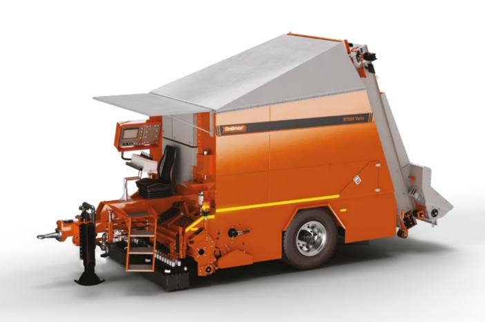
Strassmayr R 4000 is a machine assembled on a single-axle trailer designed to perform large or partial road surface repairs using emulsion and aggregate technology. The whole process of reparation is controlled by a computer, ensuring even distribution of both materials depending on the speed of the carrier truck.
