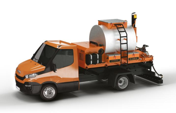
Strassmayr TS EF series sprayers come in two tank sizes: 1,5 m<sup>3</sup> and 2,5 m<sup>3</sup>. Those middle-sized units are prepared to be mounted on small trucks. Easy operation allows to quickly and precisely cover large areas with emulsion. Emulsion is kept in an isolated tank and automatically heated by a light oil burner controlled by a thermostat.
