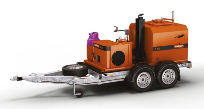
The Strassmayr A500 emulsion sprinkler is designed to spray small surfaces without the need to transport and heat large emulsion tanks. The operator can quickly and precisely cover even large areas by the use of a lance fitted with a cone nozzle. The gas heating system of the tank can be optionally equipped with an electronic thermostat, which automatically maintains the operation of the burner and keeps the emulsion always at the ideal working temperature range.
