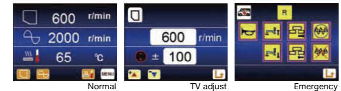
An icon is displayed on the monitor when the emergency stop button is activated.
