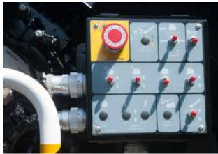
Ground level control boxes also feature improved layout and are backlit as well.
